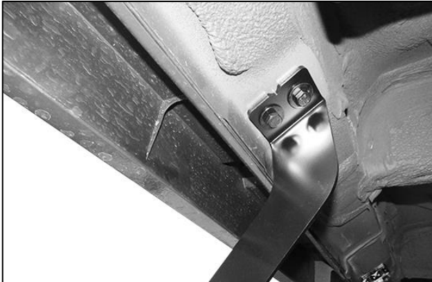
(Fig 6) (1) Passenger/Right Rear Mounting Bracket attached to the 2nd location
